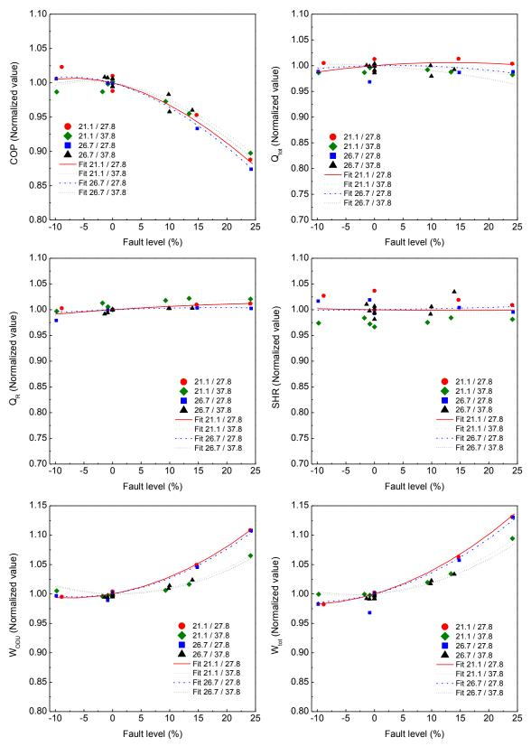
Figure 3.8. Normalized cooling performance parameters for improper electric line voltage (The numbers in the legend denote test conditions,  $T_{\text{ID}}$  (°C)/ $T_{\text{OD}}$  (°C))
