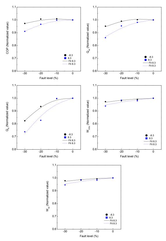
Figure 3.10. Normalized heating performance parameters for refrigerant undercharge (The number in the legend denotes *T*<sub>OD</sub> (°C))
