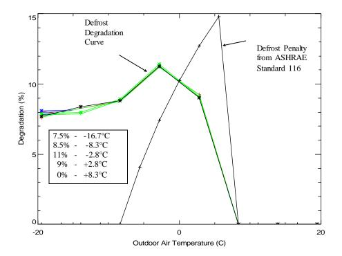
Reference for this plot is (Parker et al 1999), which is already in the back Figure 4.6. Capacity degradation due to defrost as a function of outdoor temperature (The different color lines on the plot show the defrost degradation from catalog data. The table of values summarizes the average values used in the simulations.)
