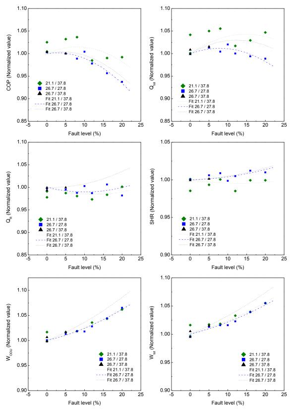
Figure 3.7. Normalized cooling performance parameters for the presence of non-condensable gas (The numbers in the legend denote test conditions,  $T_{\text{ID}}$  (°C)/ $T_{\text{OD}}$  (°C))
