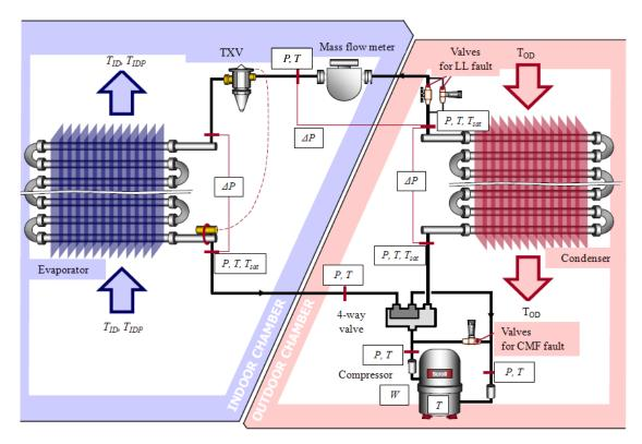
Figure 3.1. Schematic diagram of experimental apparatus (Kim et al. (2006))
