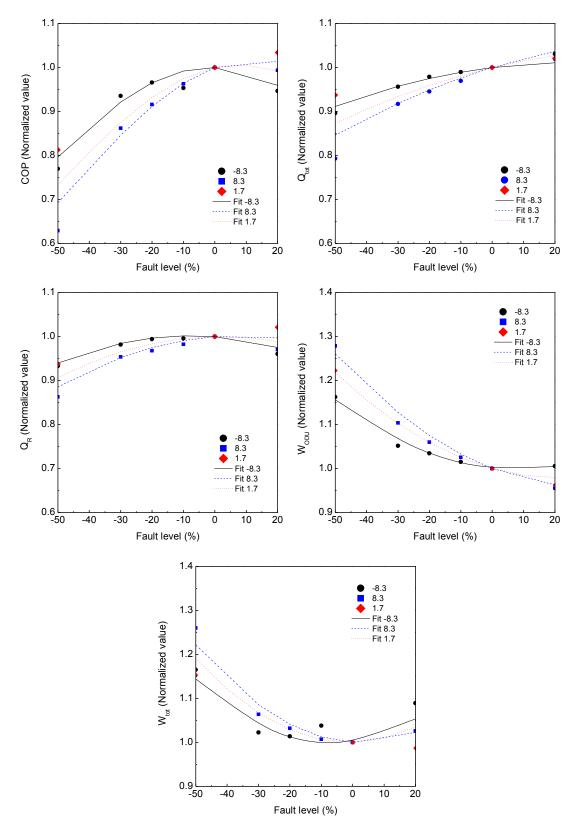
Figure 3.9. Normalized heating performance parameters for improper indoor airflow (The number in the legend denotes  $T_{OD}$  (°C))
