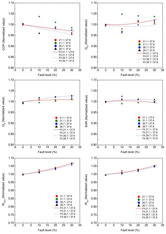
Figure 3.5. Normalized cooling performance parameters for refrigerant overcharge (The numbers in the legend denote test conditions,  $T_{\text{ID}}$  (°C)/ $T_{\text{OD}}$  (°C))
