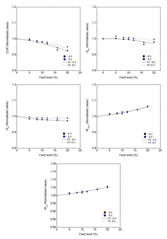
Figure 3.13. Normalized heating performance parameters for the presence of non-condensable gas (The number in the legend denotes  $T_{OD}$  (°C))
