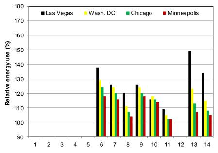
Figure 5.13. Annual energy use for houses with basement with 8 dual-fault installations referenced to the energy use for the houses with fault-free installations
