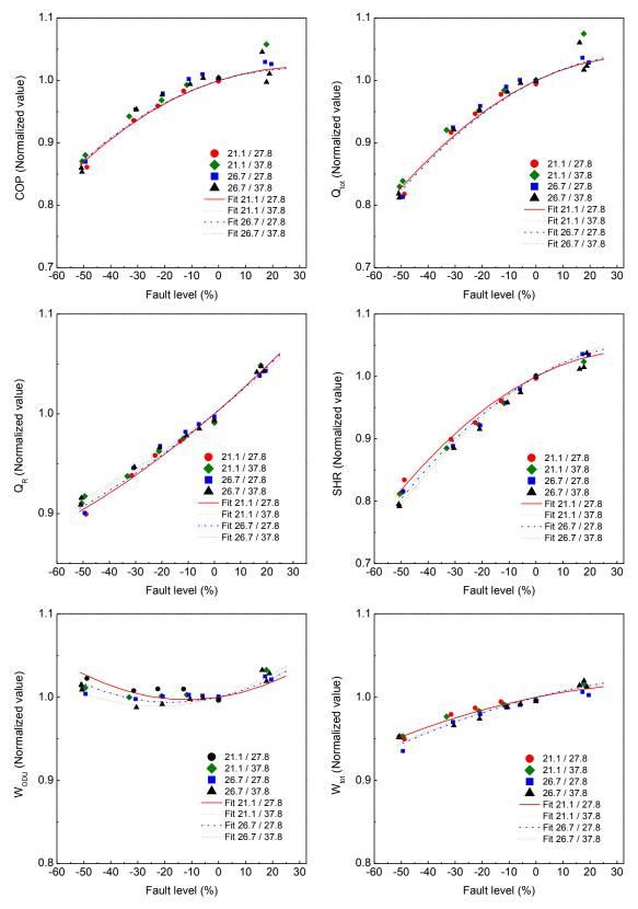
Figure 3.3. Normalized cooling performance parameters for improper indoor airflow (The numbers in the legend denote test conditions,  $T_{\text{ID}}$  (°C)/ $T_{\text{OD}}$  (°C))
