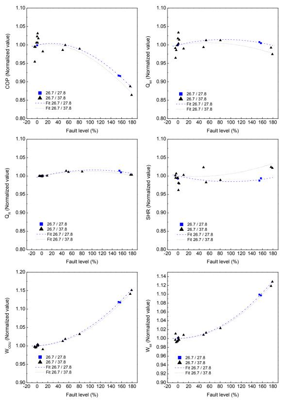
Figure 3.6. Normalized cooling performance parameters for improper liquid line refrigerant subcooling (The numbers in the legend denote test conditions,  $T_{\text{ID}}$  (°C)/ $T_{\text{OD}}$  (°C))
