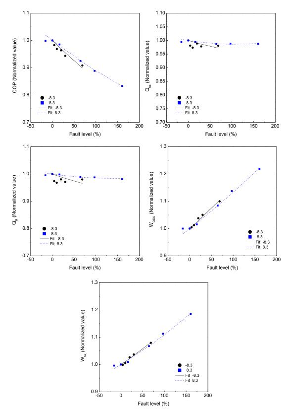
Figure 3.12. Normalized heating performance parameters for improper refrigerant subcooling (The number in the legend denotes  $T_{OD}$  (°C))
