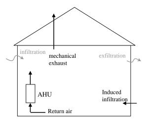
Figure 4.5. Schematic of a mechanical exhaust system
