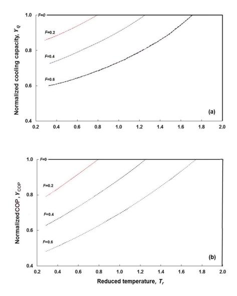
Figure 3.2. Normalized performance parameters for the cooling mode TXV undersizing fault: (a) capacity, (b) COP
