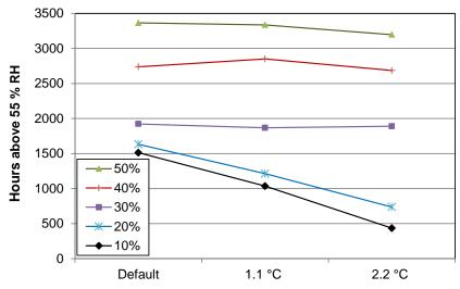
Figure 5.3. Number of hours above 55 % relative humidity for a slab-on-grade house in Houston with duct leak rates from 10 % to 50 % at three thermostat set point temperatures
