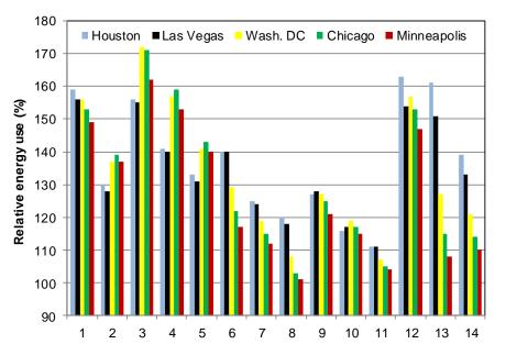
Figure 5.12. Annual energy use for slab-on-grade houses with 14 dual-faults relative to the energy use for the houses with fault-free installations
