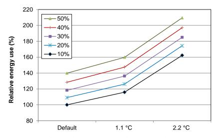
Figure 5.4. Energy use for a slab-on-grade house in Houston with duct leak rates from 10 % to 50 % at three thermostat set point temperatures related to energy use for the house at the default set point and 10 % leak rate (shown in Table 5.9)
