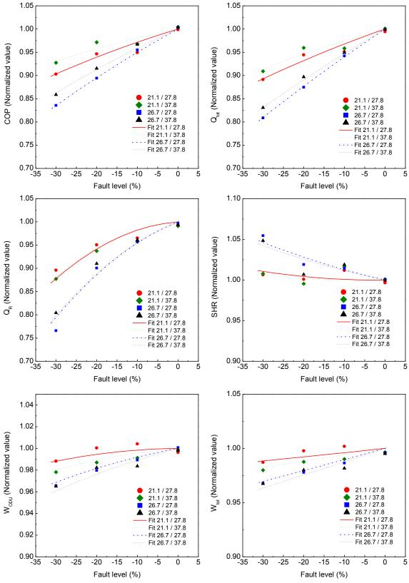
Figure 3.4. Normalized cooling performance parameters for refrigerant undercharge (The numbers in the legend denote test conditions,  $T_{\text{ID}}$  (°C)/ $T_{\text{OD}}$  (°C))
