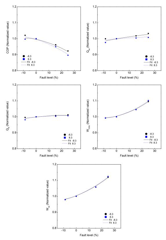
Figure 3.14. Normalized heating performance parameters for improper line voltage (The number in the legend denotes  $T_{OD}$  (°C))
