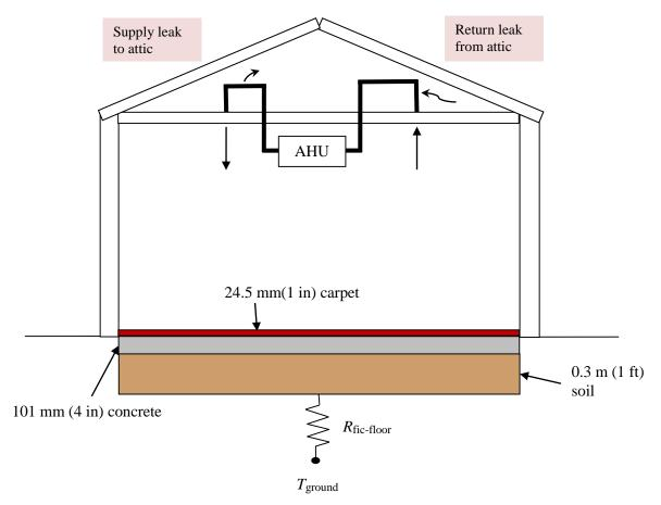
Figure 4.3. Schematic of a slab-on-grade house (ducts located in the unconditioned attic)
