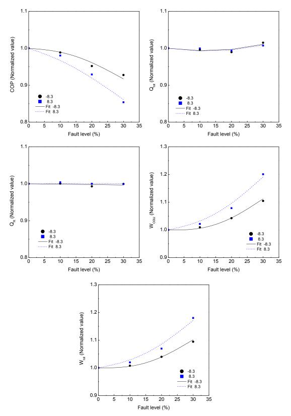
Figure 3.11. Normalized heating performance parameters for refrigerant overcharge (The number in the legend denotes *T*<sub>OD</sub> (°C))
